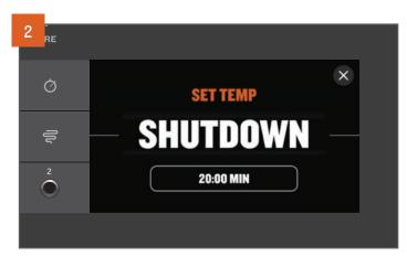
While setting the temperature, turn the selection dial all the way to the left and push to select SHUTDOWN.
