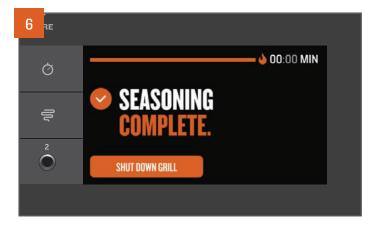
When the seasoning cycle is finished, the controller will initiate a full shutdown cycle. Shutdown cycles prevent future adverse effects and get your grill properly set up for the next cook.
