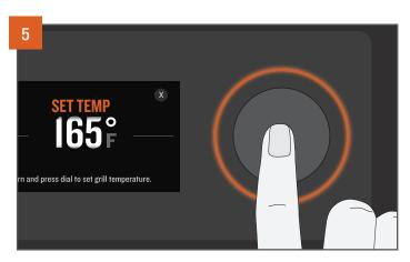
Press the center of the selection dial to select that temperature.
