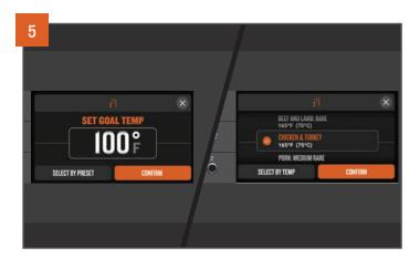
Use the selection dial to select the desired temperature for your probe goal alarm and press the dial to select and confirm. Can't remember the safe internal temperature for Chicken Marsala? Tap SELECT BY PRESET to find a list of the food-safe temperatures associated with typical protein choices.
